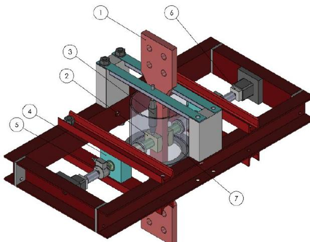
FIGURE 2 | EXPERIMENTAL TEST SET-UP FRETTING FATIGUE TESTS: 1 SPECIMEN; 2 FRETTING PAD; 3 LOAD CELL; 4 BEARING SUPPORT; 5 LOAD CELL 6 AIR CYLINDER; 7 WATER TANK
