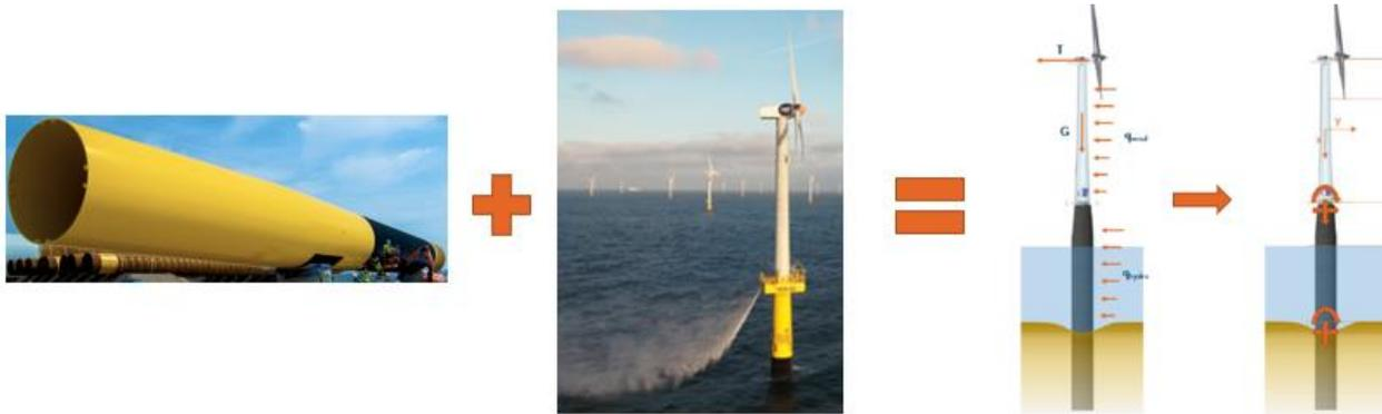
FIGURE 3 | MONOPILE FOUNDATION (LEFT) + OPERATIONAL HYDRAULIC DOT WIND TURBINE (MIDDLE) = (SIGNIFICANT) TEST LOADS (RIGHT 2X) ON THE SLIP JOINT CONNECTION
