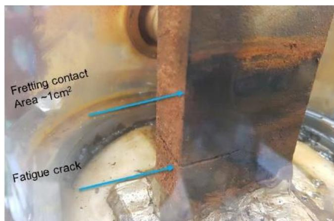
FIGURE 4 | EXAMPLE OF SPECIMEN FRACTURE
