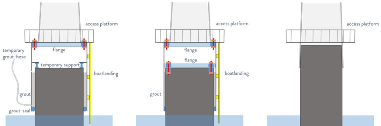
FIGURE 1 | SCHEMATIC REPRESENTATION OF A GROUTED (LEFT), BOLTED (MIDDLE) AND SLIP JOINT (RIGHT) CONNECTION
